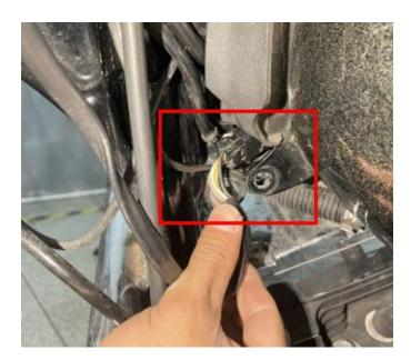
5. Unscrew the screws that fix the headlights and remove the original lights.
