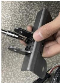
4. First remove the vehicle cushion and the screws below the fuel tank (screws do not have to be completely unscrewed, loosening can be), the screws below the fuel tank is the original light harness plug-in place, disconnect the plug-in.
