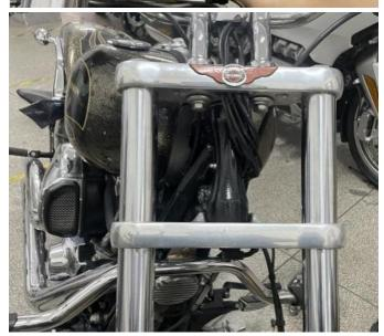
6. Unscrew the screw under the handle of the car head (when unloading the screw, you must unload it on one side, and then unload the other side of the screw after installation), the unloaded screw is connected to the pre-assembled headlight bracket in series, and then screwed back to the original place.
