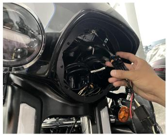
2. Unscrew the frame on the original headlight bracket, put the new headlight on the bracket,
