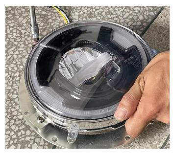
3. Put the headlight with the bracket installed back on the motorcycle, reconnect the wiring harness connector, and install the headlight decorative frame, as shown in the picture:
