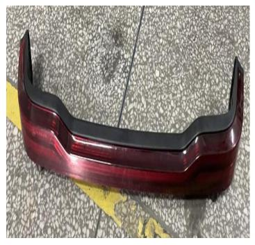
2. Open the trunk of the original car, take out the inner village, remove the original tail light, then remove the antenna and other screw accessories, and finally re-install it on the new tail light. as the picture shows:
