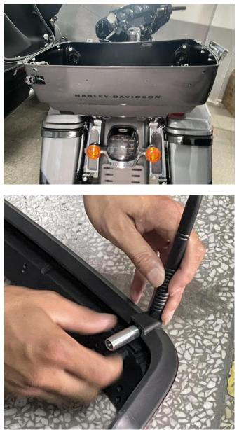
3. Put the new taillights back on the original car, and install the taillight harness connectors in advance. Tighten the screws in the order indicated in the picture (do not overtighten the screws first, and then tighten them after all the three screws are fixed). As shown in the figure:
