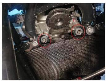
3. Clamp the two ends of the water tank protective cover into the rubber parts of the frame, and fix the upper end of the water tank with the two removed screws. The installation is complete.
