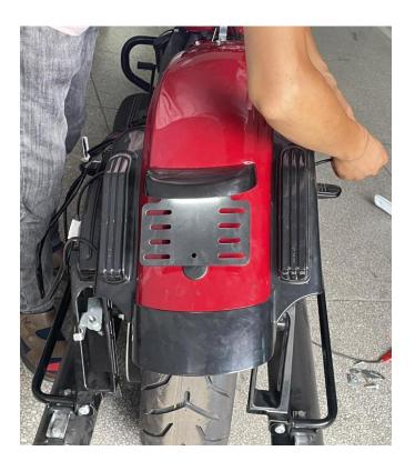
6. Follow the picture, if the original vehicle antenna is installed on the rear of the vehicle, you need to grind an arc at the edge of the taillight before screwing the antenna back on. (The arc please refer to the hole template picture. first, cut out the template paper. Then, paste it on the place where the hole needs to be opened. Finally use a polisher to follow the line make a hole). If the antenna in other positions, can be ignored this step. As shown:
