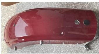
4. Install the license plate light bracket with lights and the tail lights on both sides to the fender. (Put the wire harness through the rubber plug before installation). As shown:
