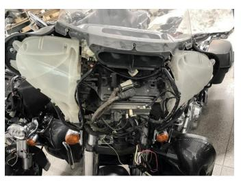
3. Find the anchor point reserved on the original fairing, then take out the template paper in the package (need to distinguish between left and right), align the center hole on the paper with the original positioning hole, and then use a 10mm drill bit to drill (need to drill at an oblique angle from the outside to the inside), and then use a 4mm drill bit to drill the rest of the 2 anchor holes.
