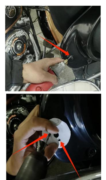
4. Finally, put the screws on the back of the mirror through the center hole just drilled, then put the nylon base over the screws, lock the nut, and use the same way to install the other side, and then install the original fairing cover as well as the windshield after both sides are installed... As the picture shows:
