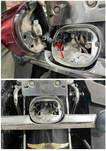
3. Unscrew the screws on both sides of the LED taillight and remove the back shell.
