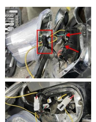
6. Tidy up the connected adapter wires, then fix the taillight.
