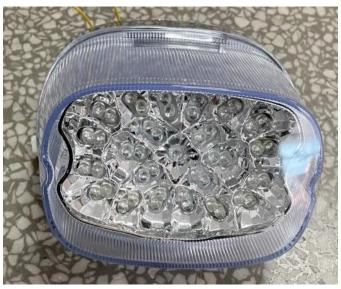
2. First unscrew the two screws fixing the original taillight for standby, unplug the harness plug-in and remove the original taillight.
