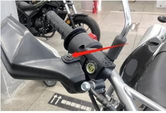
4. Installation steps for the left handguard: Referring to the installation method in step 2, simply replace the cylindrical liner with a shorter one. And the cushion block at the fixed hole below the guard can be replaced with a thick one. One end of the guard needs to be clamped at the brake coil during installation. As the picture shows:
