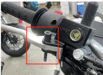
3. Installation steps for the right handguard: First, thread the cylindrical liner from the accessory package into the lower end of the brake connection screw, and then place circular pads on the upper and lower fixing holes of the hand guard. Finally, use the matching screws and nuts to fix the hand guard on the original motorcycle. (Note: The right hand guard is paired with 1 longer cylindrical liner and 2 thin cushion blocks). As the picture shows:
